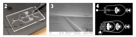
*Figure 2, left:* Acrylic microfluidic device aimed at exposing and separating the COCs. *Figure 3, middle:* SEM image of the SU-8 reversible vacuum design. *Figure 4, right:* Mask designs for microfluidic hydrogel particle maker.
