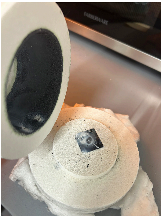
Figure 4: The alumina crucible is lined with SiC and goes inside of a 1 kW microwave.
