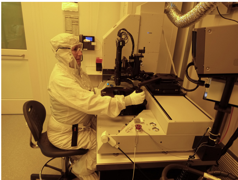
Figure 1: Ellis at the ABM Contact Mask Aligner.
