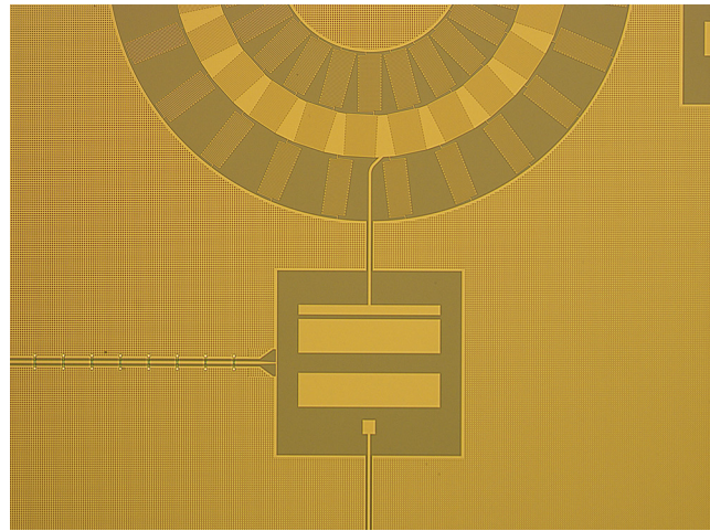
Figure 2: Zoomed-in optical micrograph of transmon qubit coupled to metamaterial ring resonator.
