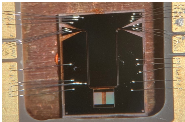
Figure 2: The LC resonator device bonded to a chip carrier.
