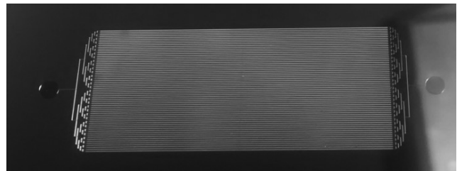
Figure 3: Etched silicon mold for hot pressing.
