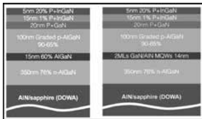
Figure 1: Schematic structures of the UV LEDs grown in this study. On the left is the AlGaIn active region LED, and on the right is the ultra-thin GaN active region LED. The AlGaIn LED has one single quantum well, while the ultra thin GaN LED has 4 quantum wells separated by 2 nm AlN barriers.
