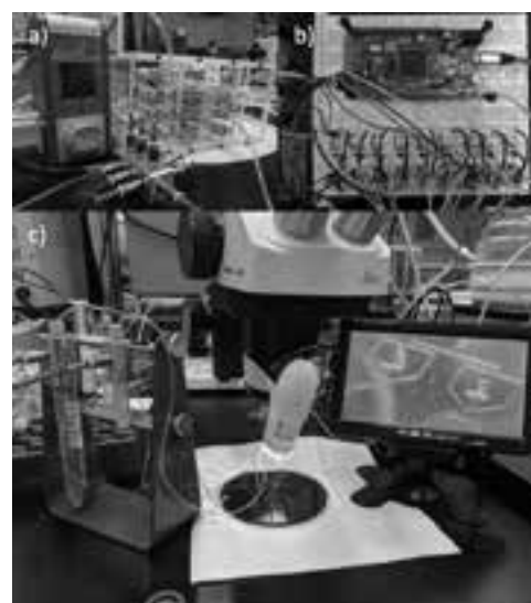
Figure 1: Equipment set-up for testing microfluidic devices. Figure 1a shows the magnetic valves and also the Fluigent pump. Figure 1b shows the Arduino microcontroller controlling the magnetic valves. Figure 1c shows the observation deck for the microfluidic devices.
