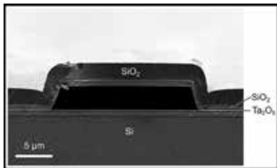
Figure 2: An SEM image of the hollow core structure after aqua regia etching.
