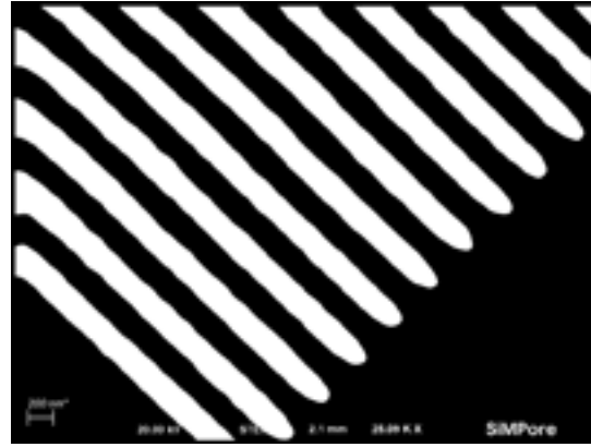
Figure 2: 25kX magnification STEM of 200 nm slits with 1:1 pitch.
