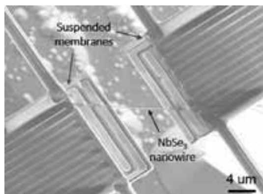
Figure 2: An SEM micrograph of an individual 135 nm-diameter \text{NbSe}_3 nanowire placed between the two suspended membranes.
