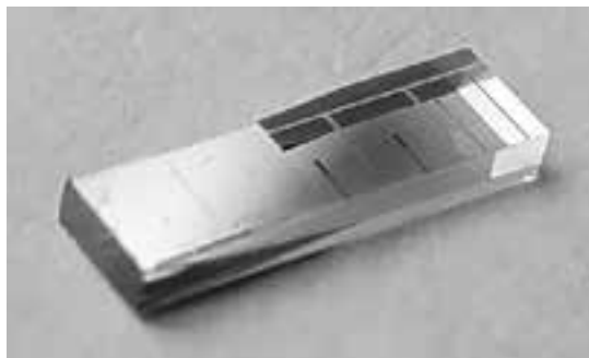
Figure 3: Diced fused silica die with patterned Al reflectors on both sides in addition to the nanophotonic pattern.
