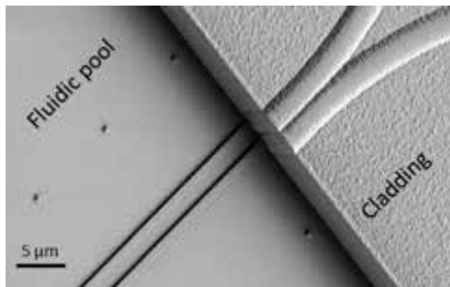
Figure 1: A tilted-angle SEM image of the step boundary of the fluidic pool region. Inside the fluidic pool region, the two parallel Si 3 N 4 waveguides trap two arrays of polystyrene microbeads (380 nm diameter) with DNA molecules tethered in between. The dot arrays near the parallel waveguides are fiducial markers for local position tracking.
