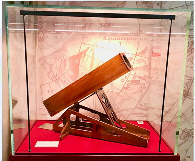
Figure 2: Foucault/Secretan, Serial No. 4: one of the first silver-coated primary mirror reflector telescopes.
