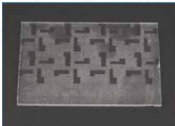
Figure 1: Thin polymer (254 \mu m thickness) was cut on the VersaLaser to yield sharp corners and ultrathin shadow profiles for use as a shadow masks. Laser jobs were run in a matter of minutes per mask with excellent reproducibility of features. Alignment and mounting holes were cut for aligning to other mask designs. (A) Kapton ® mask for use in ITO sputter deposition tool. (B) Kapton ® mask (black underside) mounted in a metal holder (made in the Clark Hall machine shop) for use in thermal evaporation for placing metal contacts.
