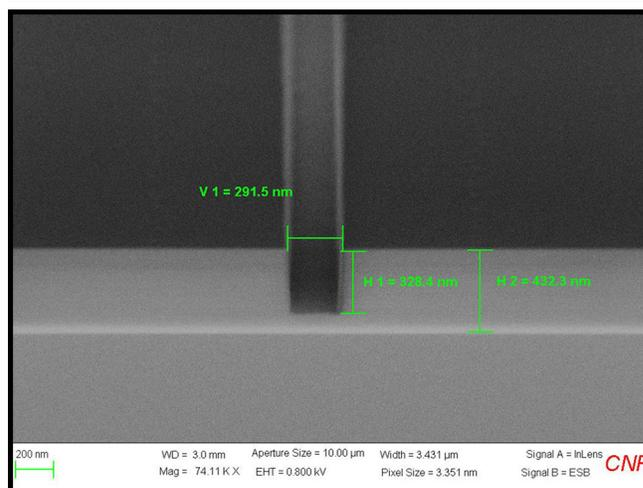
Figure 2: 300 nm silicon dioxide line etched with C<sub>3</sub>H<sub>2</sub>F<sub>4</sub> for 120 seconds. The photoresist was stripped. SEM image was taken at a 70-degree angle. The actual SiO<sub>2</sub> calculated thicknesses are approximately Height #1 = 348 nm and Height #2 = 458 nm.
