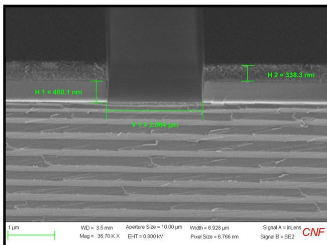
Figure 1: 2000 nm silicon dioxide line etched with C<sub>3</sub>H<sub>2</sub>F<sub>4</sub> for 160 seconds. SEM image was taken at a 70-degree angle. The actual calculated thicknesses are approximately Height #1 (SiO<sub>2</sub>) = 487nm and Height #2 (Photoresist) = 359 nm.
