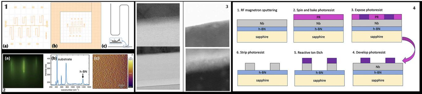
Figure 1: Device mask design. (a) Original 7.5 x 7.5 mm design. (b) Modified 6 x 6 mm design with border for alignment. (c) A single superconducting resonator with gap width  $g$  and conductor width  $s$ . Diagram from Kopas, et al. [2]. Figure 2: (a) Electron diffraction pattern, (b) Raman spectra, and (c) AFM map of hBN thin film. Figure 3: TEM of Nb sputter at 400W (left) and 50W (right) on hBN thin film. Figure 4: Complete fabrication process.
