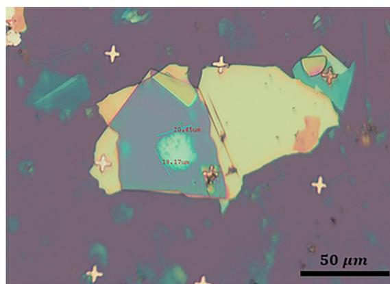
Figure 3: Optical Microscope Image of Compressed InBi Stack.
