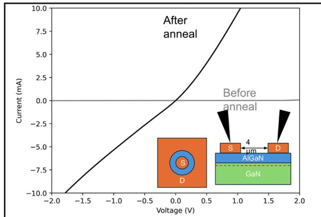
Figure 4: TLM Measurement for 800°C GaN Sample.
