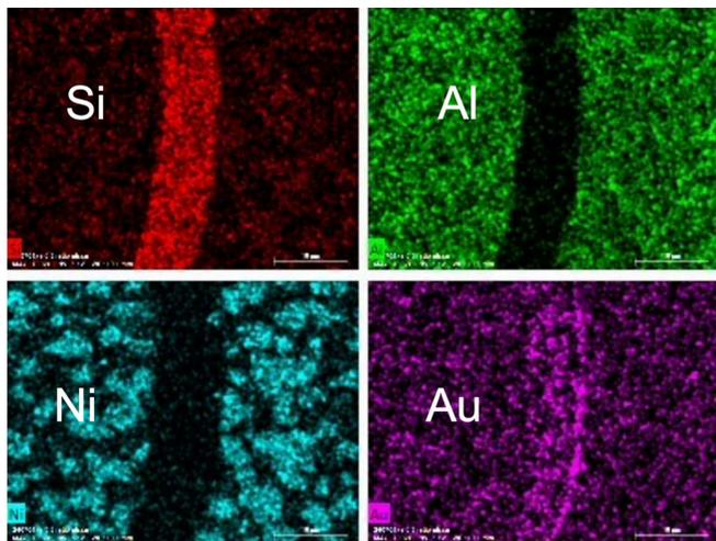
Figure 2: Si Sample 2  $\mu\text{m}$  Gap Annealed at 700°C.
