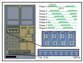
Figure 2: Optical micrograph of clockbot's integrated circuit showing the output pins for the eight phase-shifted square waves and the pins for selecting the output wave frequency. Scale bar is  $20 \,\mu m$ .
