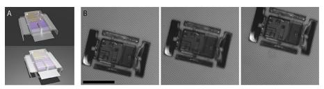
Figure 4: (A) Schematic of a CMOS integrated microscopic robot. The robot moves autonomously when powered by light. (B) A released microscopic robot walking on a glass substrate. Scale bar is  $100 \,\mu m$ .
