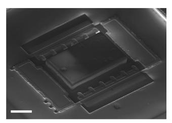
Figure 3: A scanning electron microscope image of a completed microscopic robot. The body of the robot, containing the photovoltaics and circuit, is about 15  $\mu$ m tall. Scale bar is 30  $\mu$ m.
