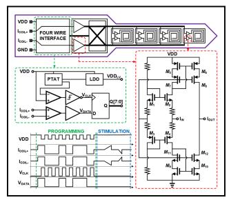
Figure 1: Circuit implementation of the proposed neural probe.
