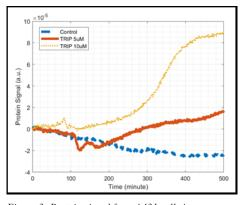
Figure 3: Protein signal from A431 cells in response to TRIP treatment. Infrared spectra collected in realtime are analyzed with principal component analysis (PCA). The spectral features at amide I and amide II absorption peaks are captured by the first principal component, the score from which is shown as the protein signal. The +y direction corresponds to a decrease in protein signal from cells.
