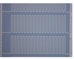
Figure 2: Optical micrograph of Nb meander-line inductor on superconducting metamaterial transmission line resonator.
