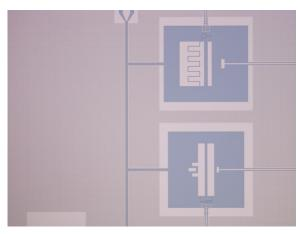
Figure 3: Optical micrograph of superconducting qubits coupled to metamaterial transmission line resonator fabricated from Nb thin film on Si.
