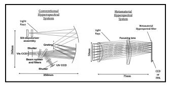
Figure 1: Phoebus's Metamaterial Spectrometer (MS) technology (right) eliminates much of the size and weight of conventional hyperspectral spectrometer technologies (left). Note the significant difference in scale of the two images.
