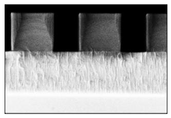
Figure 4: SEM image (cross section) of etched pillars with near-vertical sidewalls. Imaged at ~ 90 kX in the Zeiss Supra SEM, the grain structure of the etch stop layer is clearly visible.
