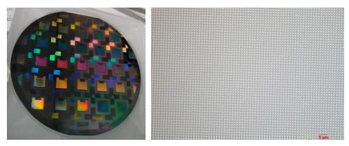
Figure 2, left: Wafer lithographically patterned with optical metastructures, using the ASML DUV stepper, Figure 3, right: Optical microscope image of test pattern of array of ~ 1  $\mu$ m pillars, also patterned on the ASML.
