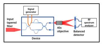
*Figure 3: Illustration of testing setup.*
