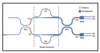
Figure 1: Layout of the device with heaters (not to scale). DC: directional coupler; H: heater; MMI: multi-mode interferometer; O: output.
