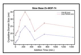
Figure 2: Average crystalline domain sizes of Zn-MOF-74 crystallites prepared by slow addition of base.
