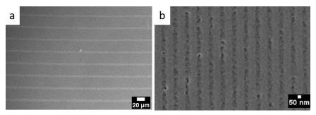
Figure 2: (a) Line pattern measured using scanning electron microscopy; (a) after DUV exposure on an ASML PAS 5500/300C DUV wafer stepper ( $\sim$  40 mJ/cm²), feature size 1  $\mu$ m, (b) after exposure on a JEOL 6300 to 75  $\mu$ C/cm² e-beam radiation. The feature size is 50 nm.
