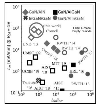
Figure 1: Current-levels and modulation ratios achieved for various p-channel device demonstrations in the III-Nitrides. Noting that this is a rapidly advancing field, it is critical to timestamp this benchmark as drawn from only the publicly available literature as of July 2019. It is seen that GaN/AIN devices enable some of the highest on-currents possible. (See pages vi-vii for full color version.)
