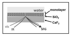
and sum-frequency generation, infrared and visible transparent  $CaF_2$  windows are coated with SiO<sub>2</sub>. Then after surface functionalization with silane monolayers, the water structure and dynamics at the interfaces can be explored with sum-frequency generation.
