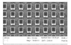
Figure 1: SEM of a typical  $\alpha$ -Si-based near-IR resonant metasurface on a SiO<sub>2</sub>/ITO substrate.
