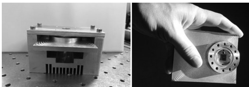
Figure 3: a) Complete Phoebus handheld biosensor system, b) removable module with plasmonic chip.
