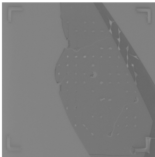
Figure 1: Optical microscopy image of a WSe 2 monolayer transferred over an array of nanopillars. Bright spots indicate tenting sites resulting in local strain in the WSe 2 monolayer.
