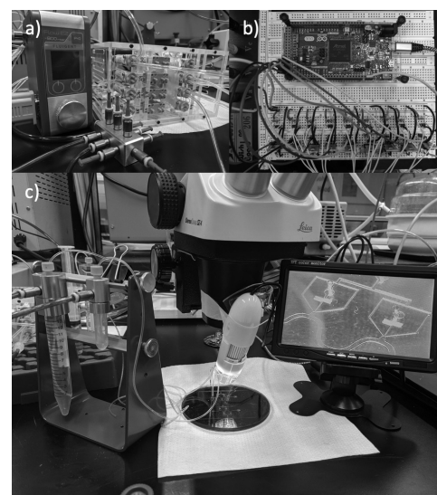
Figure 1: Equipment set-up for testing microfluidic devices. Figure 1a shows the magnetic valves and also the Fluigent pump. Figure 1b shows the Arduino microcontroller controlling the magnetic valves. Figure 1c shows the observation deck for the microfluidic devices.
