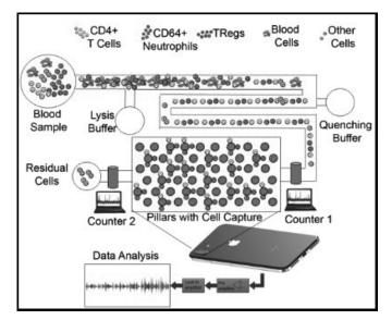
Figure 1: Schematic of microfluidic chip design.
