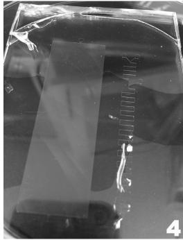
*Figure 2, top:* Deep etched silicone wafer mold. *Figure 3, middle:* Ten times magnification of silicone mold inlet to antibody capture chamber. *Figure 4, bottom:* PDMS device cast from the silicon mold.
