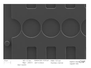
Figure 2: SEM image of a row of 1  $\mu$ m constrictions created by etching 5  $\mu$ m into silicon by deep-reactive ion etching.
