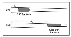
Figure 1: Bacteria under fluid pressure (p) are forced into tapered channels. The distance a cell travels into a tapered channel depends on cell stiffness with more compliant cells traveling further into the channels. The distance traveled by a cell into the tapered channel (d1) is therefore an indicator of cell stiffness. Viewing the deformation of a cell under two different applied pressures can be used to determine the mechanical properties of the cell envelope.
