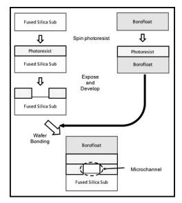
Figure 1: Process flow of fabricating side-coupled microfluidic devices.
