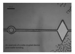
*Figure 2: Micrograph showing side-coupled microfluidic device after wafer bonding.*
