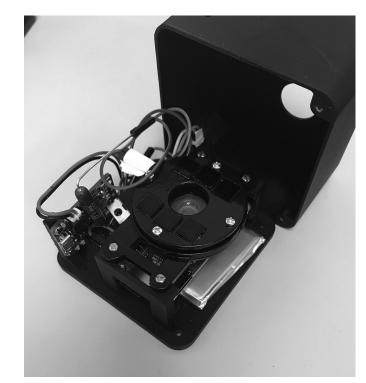
Figure 4: 3D-printed imaging device.
