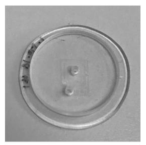
Figure 1: Image of completed microfluidic chip.
