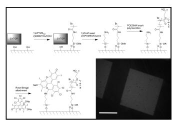
Figure 2: Process flow for the fabrication of the biosensor platform and the picture of the platform taken with a fluorescent microscope.
