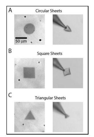
*Figure 3: Final wrapped states for various sheet geometries.*
