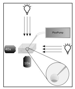
Figure 1: Schematic of setup. Inset shows Fluorinert drop with 2D material wrapping from the bottom.
