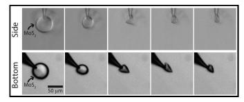
*Figure 2: (top) Time lapse of Fluorinert droplet wrapping by*  $MoS_{2^{\prime}}$  *side view; (bottom) Time lapse of the same droplet wrapping, bottom view.*
