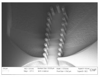
Figure 1: An image of the micropillar section of the microchannel that has been captured with a scanning electron microscope (SEM).
