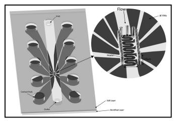
*Figure 2: Schematic illustration of microchannel, which consists of arrays of micropillars within.*
