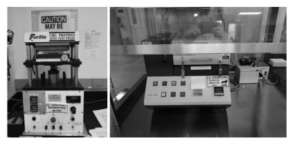
Figure 1: Hot press and UV-Ozone equipment used for making microfluidic device.
