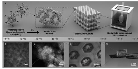
procedure. This process combines the inherent porosity of connecting PLIC units at the nanoscale and the advantage of additive manufacturing at macroscopic scale that enables conventional powder-like porous materials be constructed to intricate designed architectures unattainable with conventional fabrication schemes.
