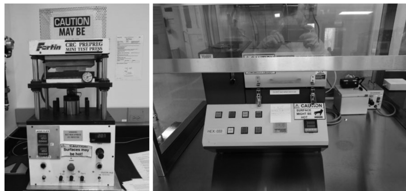
Figure 1: Hot press and UV-Ozone equipment used for making microfluidic device.
