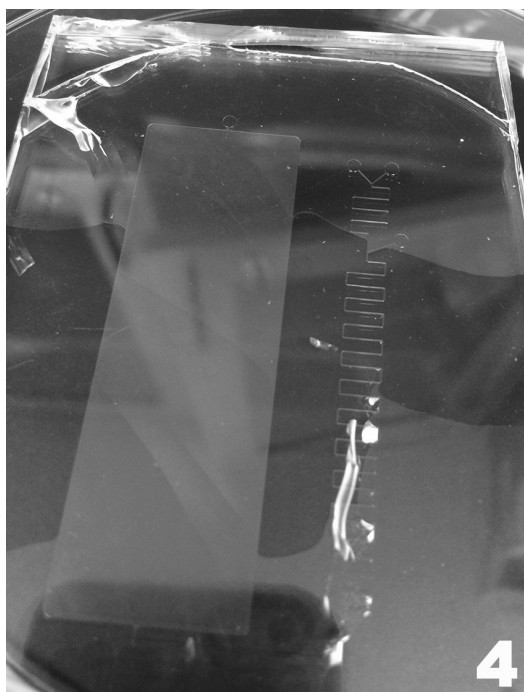
Figure 2, top: Deep etched silicone wafer mold. Figure 3, middle: Ten times magnification of silicone mold inlet to antibody capture chamber. Figure 4, bottom: PDMS device cast from the silicon mold.
