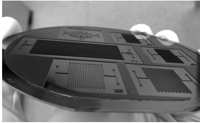
Figure 2: Wafer after being removed from Unaxis 770 deep Si etcher.
